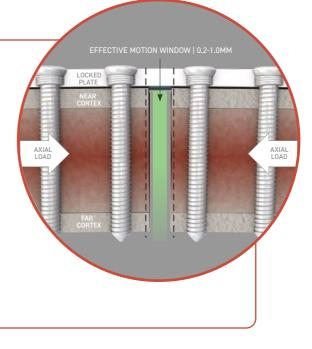
Locked plating inhibits interfragmentary motion
